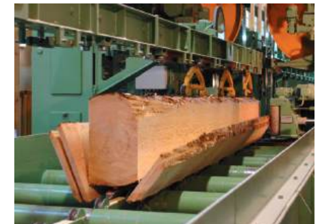
3. Sawing side boards
