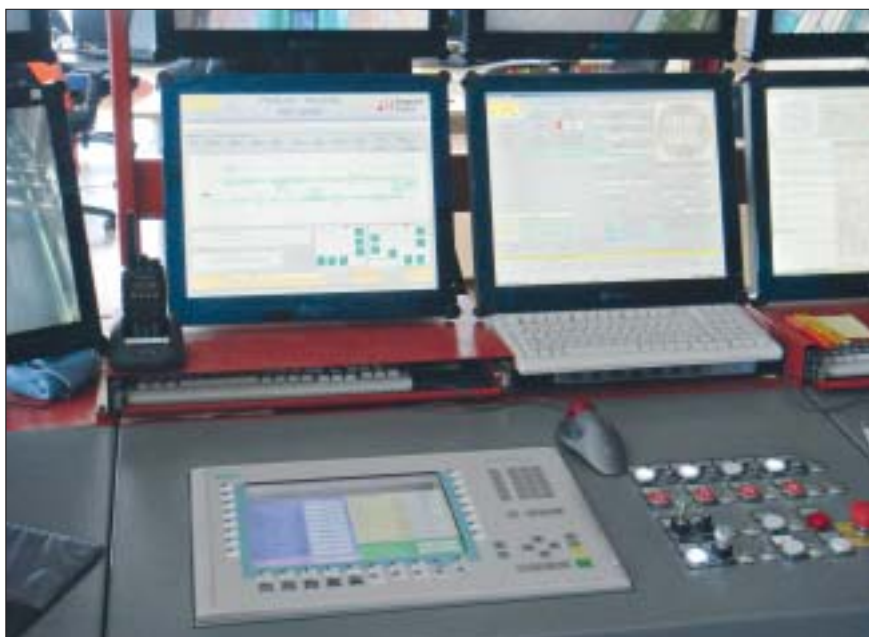
The complete “Arcoline” saw line at Bergkvist Insjön can also be controlled locally – in other words, independently of the control level – by means of the nine distributed “Simatic Multi Panels MP370” (right) installed at the main machines
