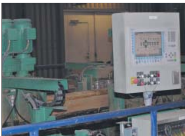
The complete “Arcoline” saw line at Bergkvist Insjön can also be controlled locally – in other words, independently of the control level – by means of the nine distributed “Simatic Multi Panels MP370” (right) installed at the main machines
