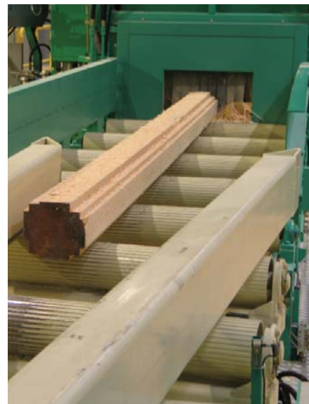
Because of the diagonal shifting function and the full optimisation process, each profiling unit replaces one full high performance edger optimiser system
