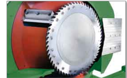
Straight knives chipper head with pre-sawing circular saw ring
