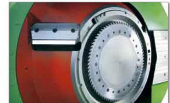
Straight knives chipper head with post-sawing circular saw ring for opening of the heads in the cut
