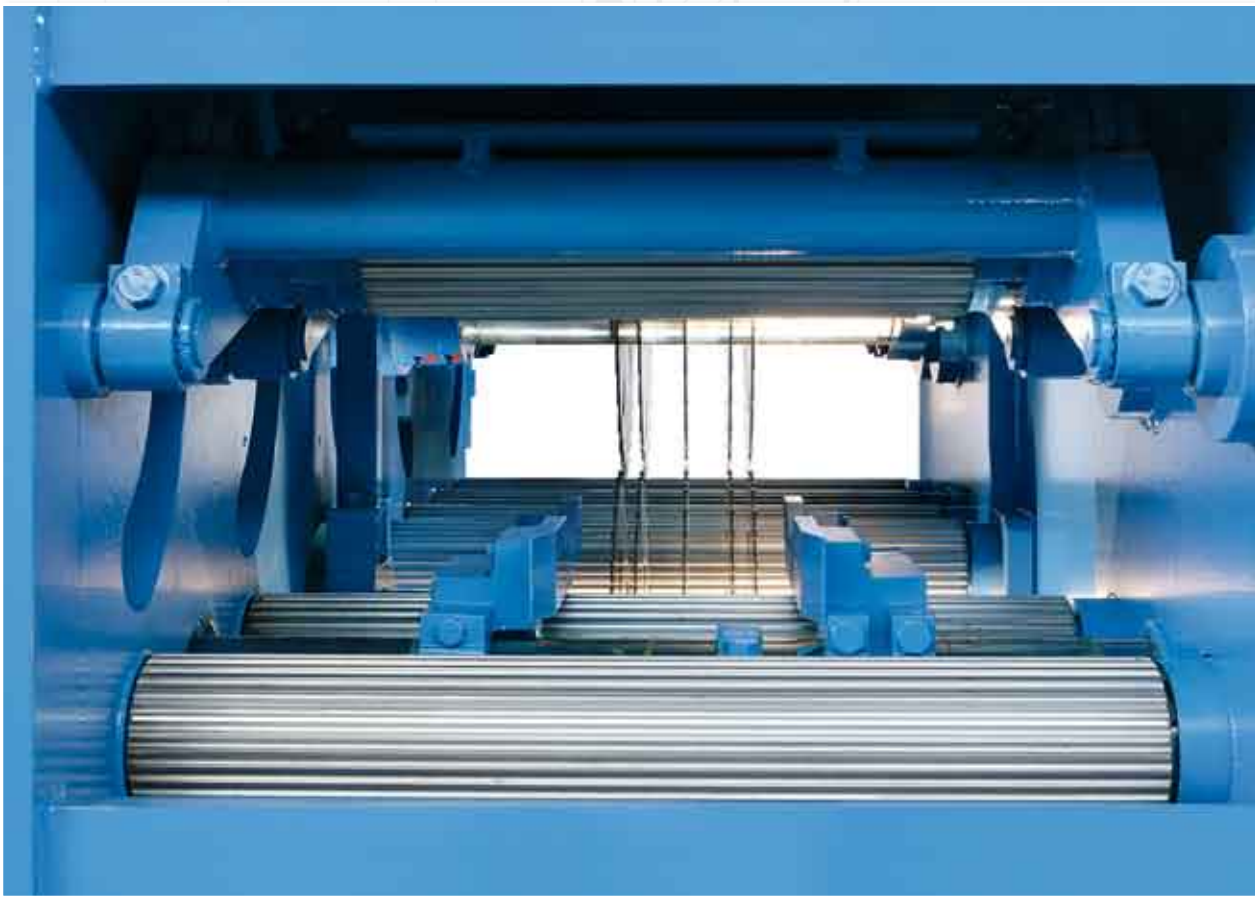
Double arbor circular resaw with fix-mounted saw blades
