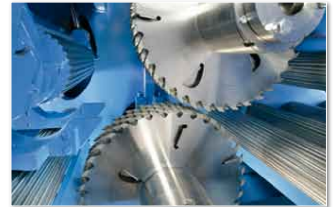
Double arbor circular saw with lumber guides
